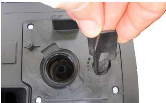
3. If necessary adjust grind coarseness with the grinder adjustment spanner.
